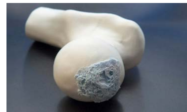
Bone mimicking structure with a 3D-printed covering of dense ceramics and a foam ceramic filling.
